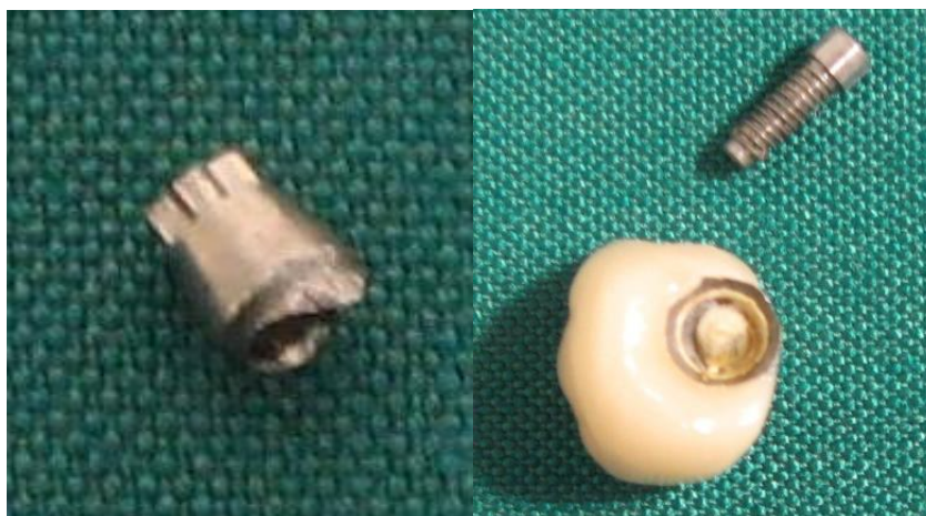
Figure 1. The fractured fragment of the abutment with the screw protective cotton within the crown
