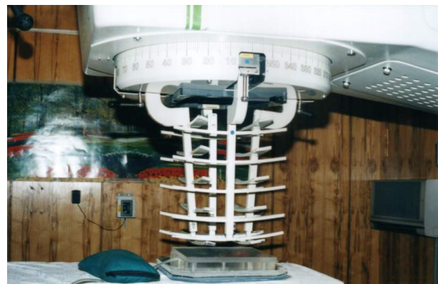
Figure 1. Dosimetry configuration of the 6 MeV electron beam by Neptun 10 linear accelerator inside the acrylic phantom
