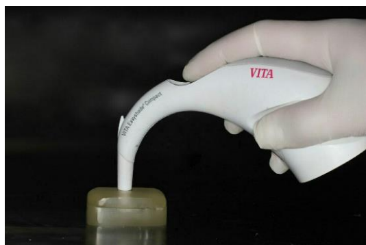
Figure 1. Measurement of color parameters under standard conditions with the sample placed in the positioning jig
