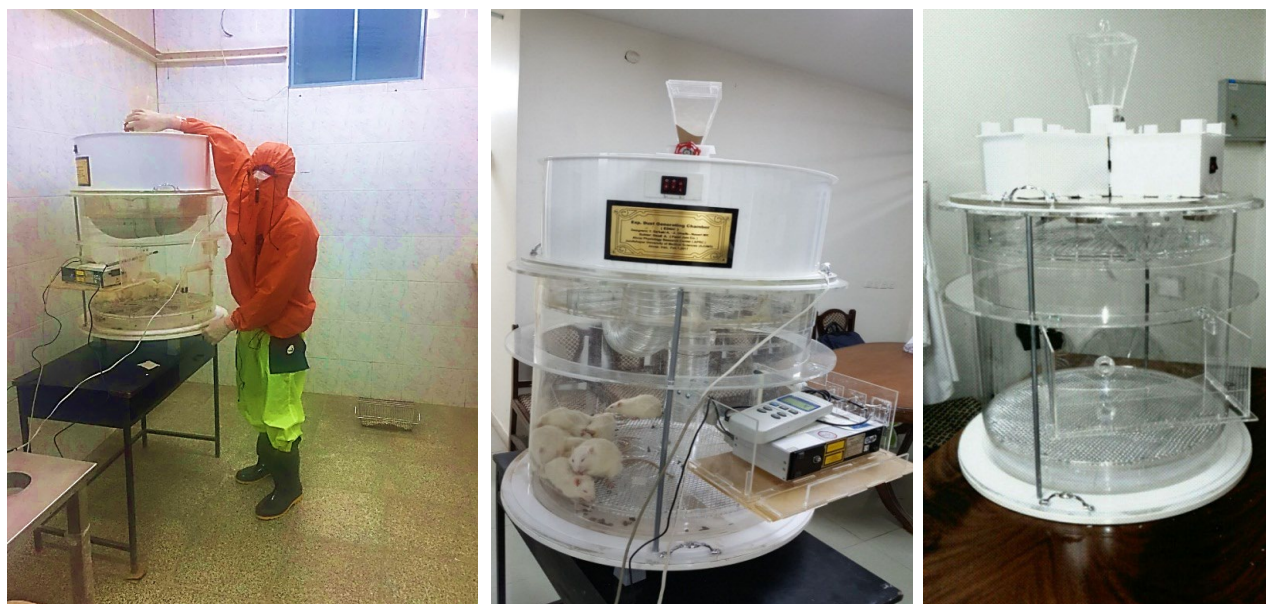
Figure 1. Designated experimental dust storm making chamber (designed by Prof. Sarkaki A., Made by Omid Iranian Co. Tehran and Aref. Jam Co. Ahvaz, Iran).
